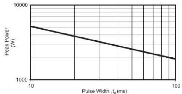
Fig. 4 - Peak Pulse Power Rating Curve
